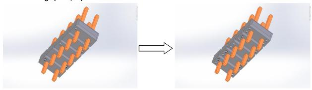
Reason for change: Improvement on the 1 & 2 positions (cut) header sit flat on the PCB.
