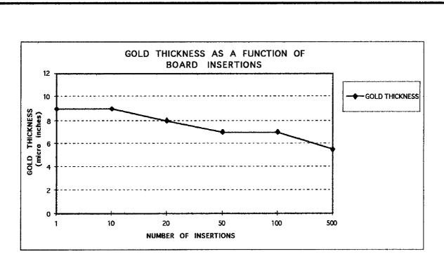
\*\*\* GOLD THICKNESS MEASURED ON CONTACT NUMBERS 24, 26, 30, 36, 38 AND 40.
