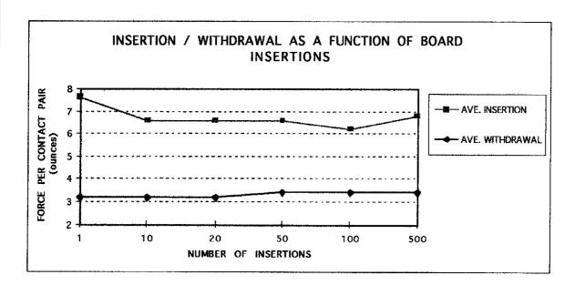
\*\*\* INSERTION / WITHDRAWAL MEASURED ON CONTACT NUMBERS 3, 4, 31, 32, 57 AND 58.
