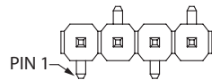
P/N: R C S D-M30RC (OPPOSITE BEND, ONLY APPLICABLE ON EVEN PIN COUNTS)
