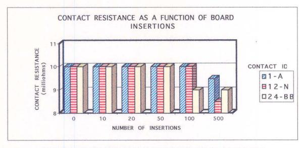
\*\* CONTACT RESISTANCE MEASURED BETWEEN PC BOARD AND CONNECTOR TERMINATIONS.
